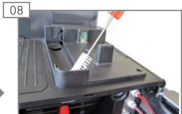
08 Clean the powder chute with a brush.
