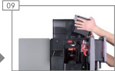
09 Attach the powder container.
